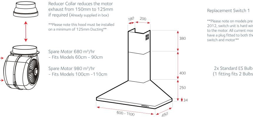
\*\*Please note on models pre 2012, switch unit is hard wired to the motor. All current models have a plug fitted to both the
